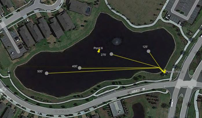
Pond Turn Calculation Surface Acres Average Depth 2.7 10 **GPM Per Air Station** 3,200 Total Pond or Lake Volume (gallons) 8,797,977 Area to be Aerated 2.7 **Average Depth of Aerated Section** 10 Volume of Water in Aerated Section (gallons) 8,797,977 System CFM Daily Operating Hours 24 # of Air Stations **CFM Per Air Station** 2.15 19,814,400 **GPM Daily** # of Daily Turns of Aerated Section 2.25
